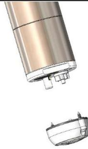
Step 2: Before separating the Sensor Cover from the sensor end, position the sensor vertically, with the wet side facing down, to prevent the balls from escaping. Pull down without twisting.
