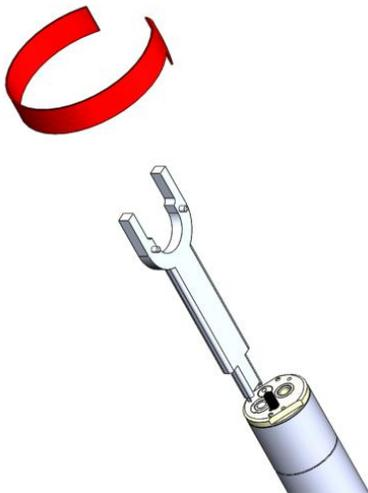
Figure 19: Unthread the sensor by twisting counterclockwise (CCW).
