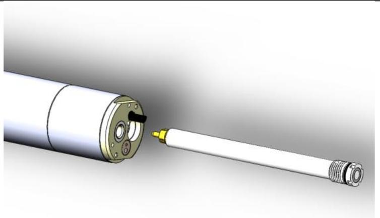
Figure 25: Remove the pH Sensor and discard. Replace with a new one. Make hole is wiped clean. Replacement sensor has silicone grease and an o-ring applied.
