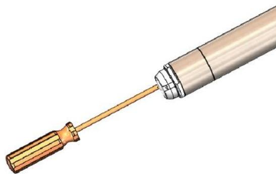
Step 9: Tighten screws until there is no gap between the Sensor Cover and the Sensor End.
