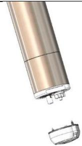
Step 8: Line up the temperature sensor and motor impeller with the holes in the sensor cover. Twist very gently until the pins on the Sensor Cover engage with the holes in the Sensor End and the Sensor Cover sits flush with the Sensor End.
