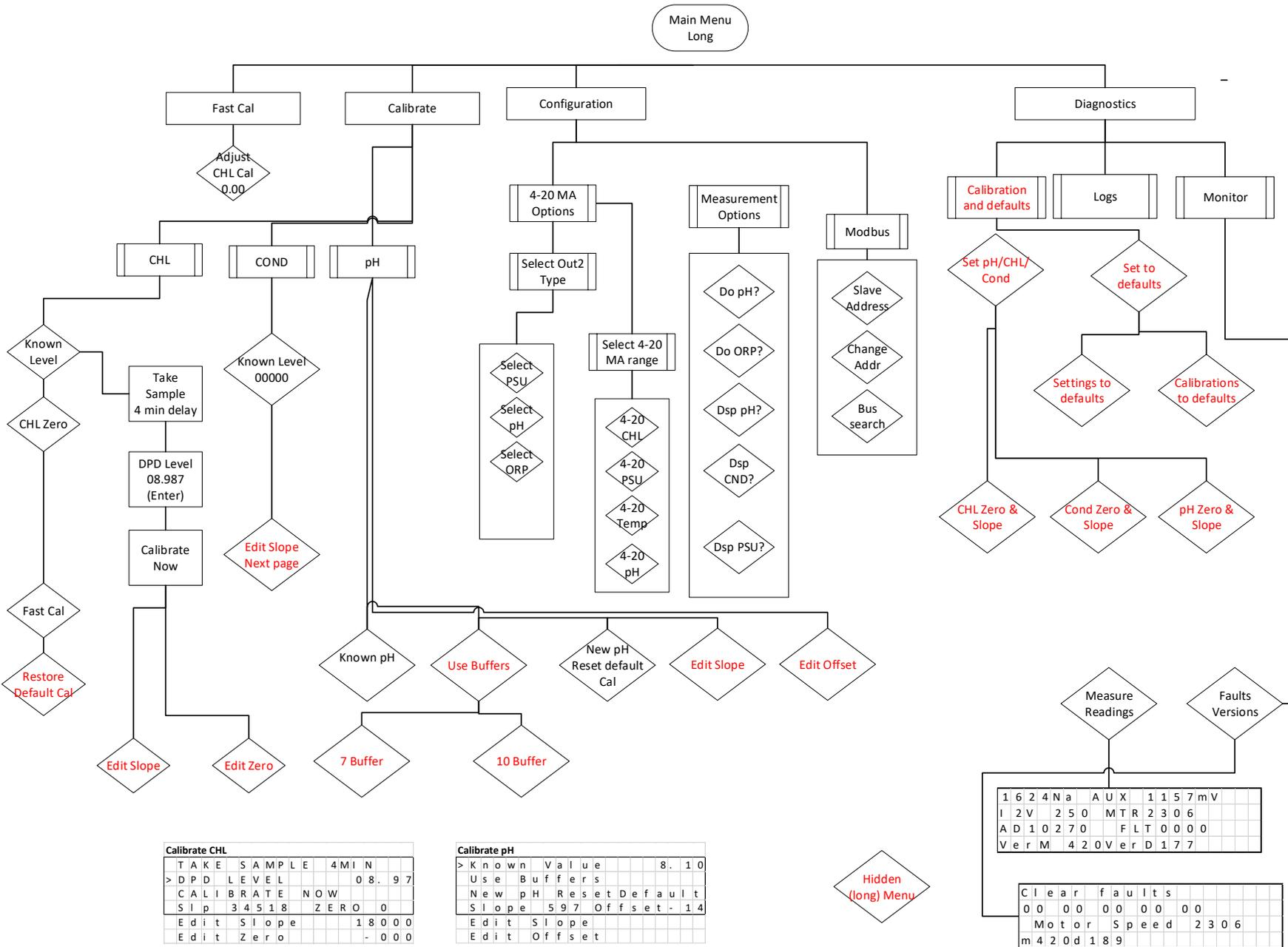
To enable the Long Menu: Press the **➔** and **SELECT** Key for at least 2 Seconds. You will see a notice that the Long Menu is Now Active. This will remain until the Display is powered off and on.
