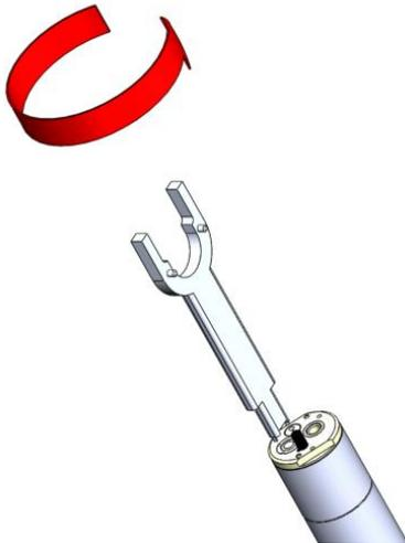
Figure 24: Unthread the sensor by twisting counterclockwise (CCW).
