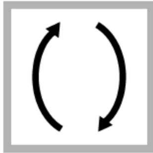
10. Close the sample cell. Invert the sample cell for about **20 seconds** to dissolve the reagent. Undissolved powder will not affect accuracy. A pink color will show if chlorine is in the sample.
