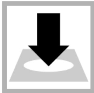
14. **Total chlorine measurement:** After 3 minutes and within 6 minutes of the reagent addition, insert the prepared sample into the cell holder. Point the triangle mark on the sample cell away from the keypad.
