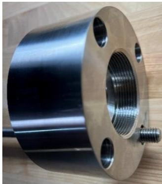
Figure 6. Valve-side of cap showing  $\frac{1}{2}$  inch protrusion of all-thread rod.
