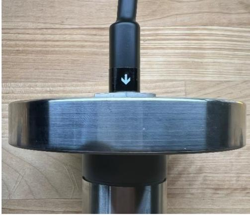
**Figure 9. Orientation arrow depicting location of ejection port on sensor end. Line up perpendicular to flow direction.**
