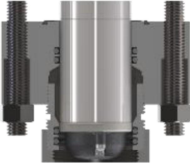
Figure 7. Cross-Section of Cap with sensor end pushed passed both internal O-rings.
