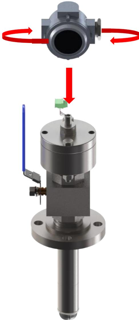
Figure 12. Junction box installation instruction.
