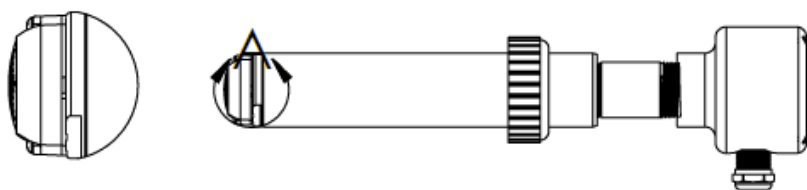
Figure 7: Outlet port orientation to ensure outlet port is "up" to purge air.
