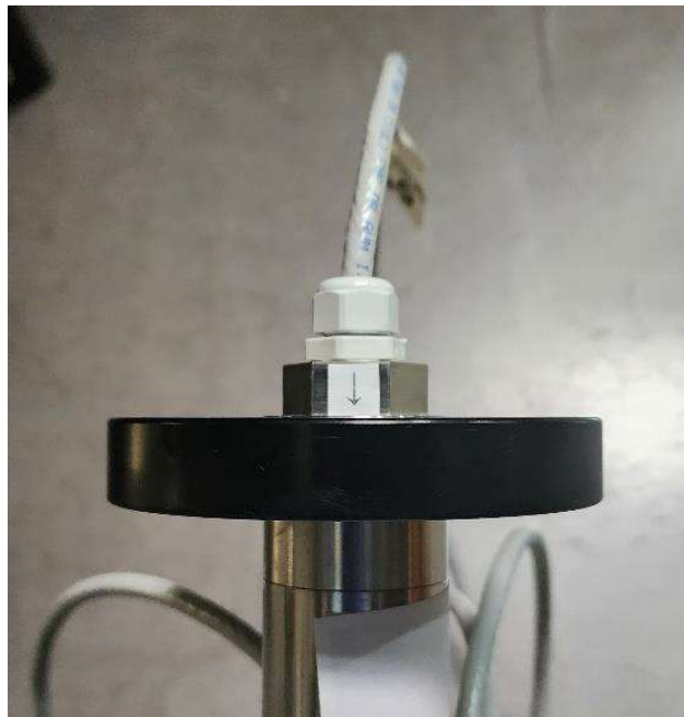
Figure 8. The outlet port aligns with the sticker shown.
