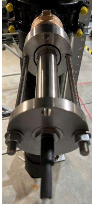
Figure 11. Orientation arrow depicting location of ejection port on sensor end. Line up perpendicular to flow direction.
