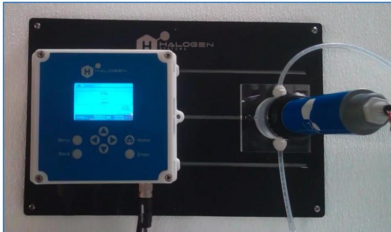
The controller shows sensor measurements and other data on the display, transmits analog and digital signals, and interacts with other devices through outputs and relays. Outputs, relays, and sensors are configured and calibrated through the user interface on the front of the controller or remotely for network-connected controllers.
