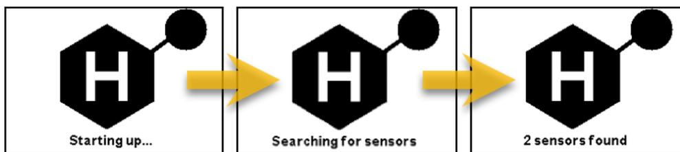
When the D20 power-up is completed, the sensor will start its start-up sequence. Once completed, all pertinent sensor information is displayed:
