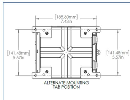
2. Attach the enclosure to the wall with the appropriate wall-mounting screws (not included) that will firmly hold the enclosure to the wall. Make sure that all four corner mounting tabs are attached.
