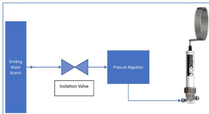
The pressure-reducing valve is needed if the supply water line pressure exceeds 60 PSI/4 Bar. The flow cell is equipped with  $\frac{1}{4}$ " *John Guest push-to-connect* (PTC) fittings on both the inlet and the outlet. A short length of tubing is supplied for each connector.
