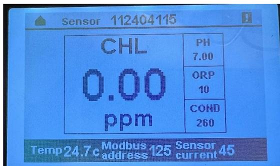
Verify all sensor values displayed on the D20. If pH requires calibration, perform that step first before continuing. Check the Chlorine level using a handheld pocket colorimeter and adjust the calibration as needed.
