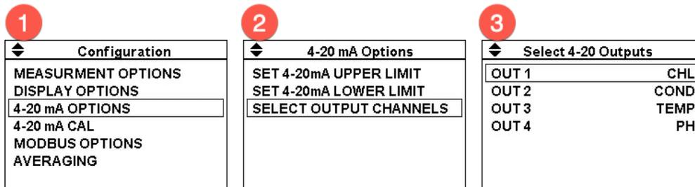
To set the scaling limits between the PLC and the D20:
