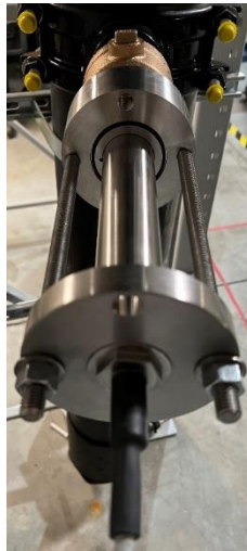
Figure 10. Orientation arrow depicting location of ejection port on sensor end. Line up perpendicular to flow direction.
