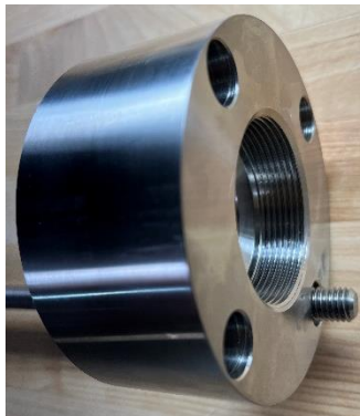
Figure 6. Valve-side of cap showing ½ inch protrusion of all-thread rod.
