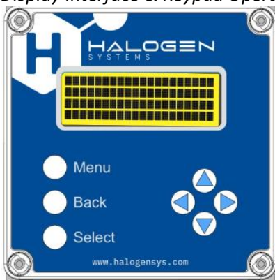
Figure 7: Main Screen: normal display after startup and sensor beginning normal operation. This screen will appear for 3 to 5 seconds
