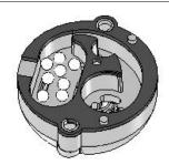
Step 7: Place the cleaning balls in the larger cavity of the new Sensor Cover as shown above. Make sure no balls are in the other (impeller) cavity.
