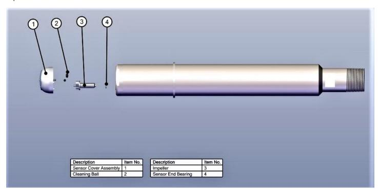
Exploded View of EX-P-HT4 and EX-P-STD/STD2
