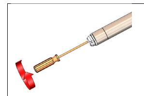
Step 1: Remove the screws holding the Sensor Cover and strainer on to the sensor end.
