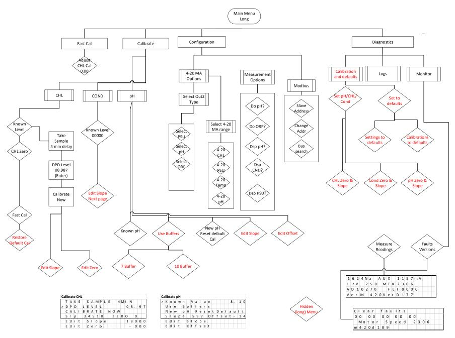
To enable the Long Menu: Press the  $\rightarrow$  and SELECT Key for at least 2 Seconds. You will see a notice that the Long Menu is Now Active. This will remain until the Display is powered off and on.
