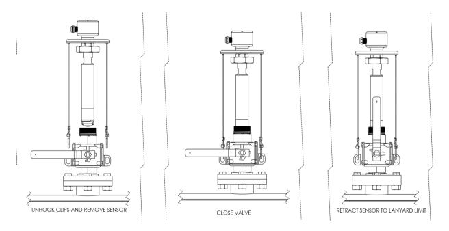
Figure 20: Remove sensor from Hot Tap Valve (Sequence Right to Left for removal)
