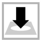
12. Free chlorine measurement: Within 1 minute of the reagent addition, insert the prepared sample into the cell holder. Point the triangle mark on the sample cell away from the keypad.
