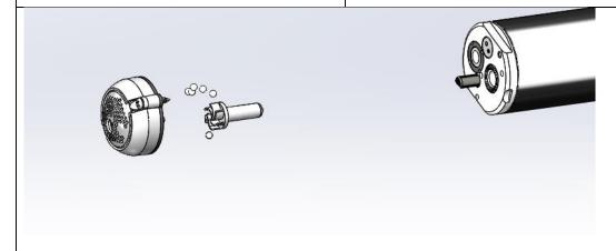
Step 3: Remove the sensor cover assembly, impeller and cleaning beads. Note which impeller was
