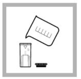
Prepare the sample: Rinse a second 1-cm/10-mL sample cell and cap three times with sample. Fill the sample cell to the 5-mL mark with sample.
