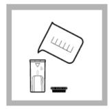
2. Prepare the blank: Rinse a 1-cm/10-mL sample cell and cap three times with sample. Fill the sample cell to the 5-mL mark with sample. Close the sample cell
