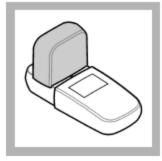
Install the instrument cap over the cell holder.
