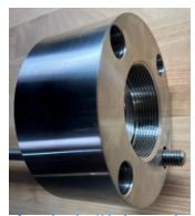
Figure 6. Valve-side of cap showing ½ inch protrusion of all-thread rod.
