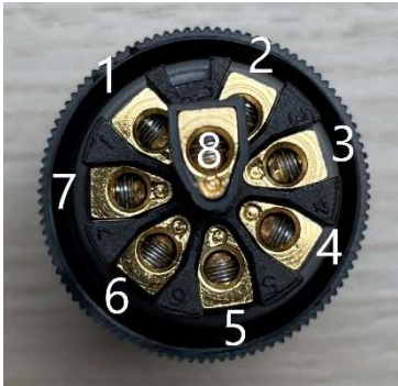
Figure 5: Pin Out for M12-8 A Code connector for 4-20 mA Outputs
