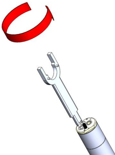
Figure 21: Unthread the sensor by twisting counterclockwise (CCW).
