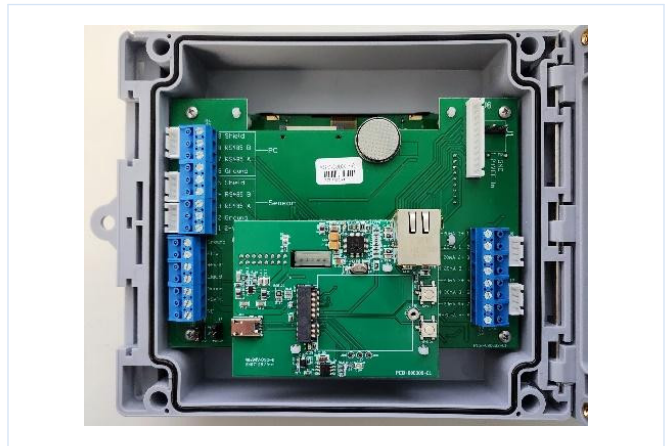
Figure 25. D20 real-time-clock battery location.
